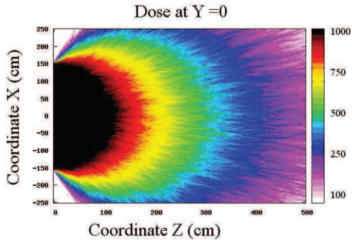
**Figure II.8.** Dose rate in the range of 100 and 1000 Sv/h produced by electrons of 10 MeV impacting in a W sheet. The cosine of the angle is 0.6.
