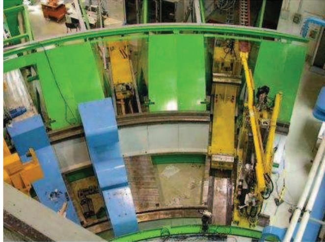
**Figure 9.9.** Area of the DTP installation showing the cassette Mover inside the vessel (yellow), the divertor model (blue) and Sector '72' of the lower region of ITER and its rails70 (green).
