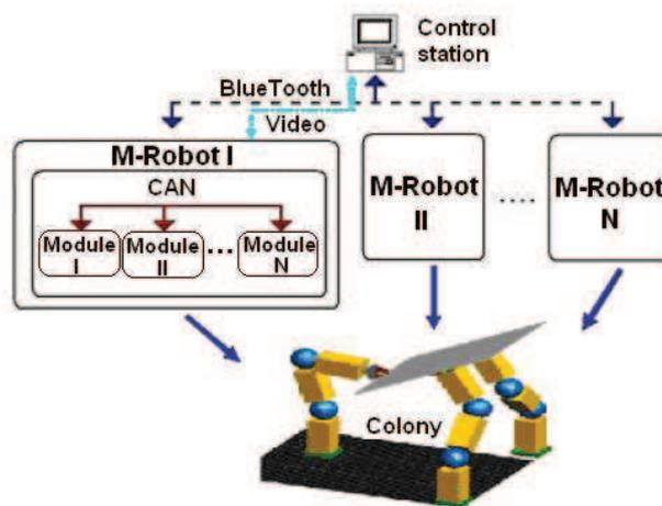
Figure 9.23. Modular system cooperating to perform tasks.
