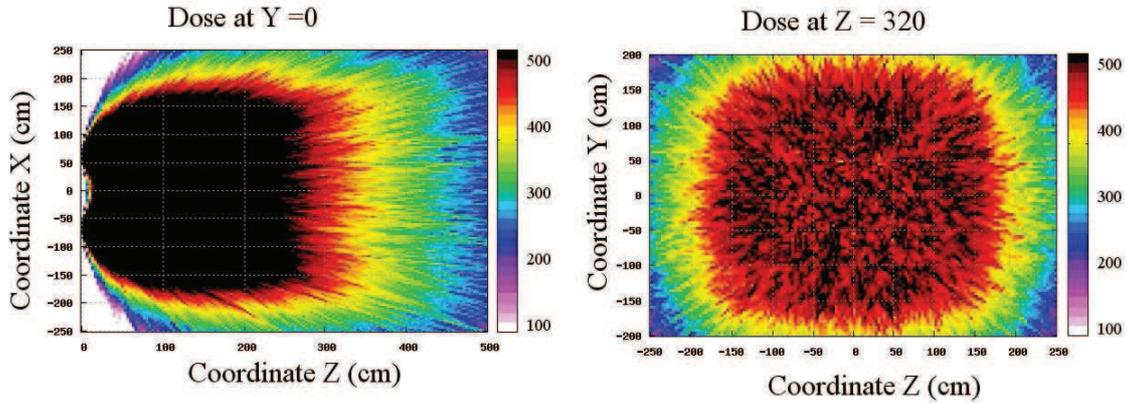
Figure II.4. Dose rate produced by electrons of 10 MeV impacting in a W sheet. The cosine of the incidence angle is 0.3.
