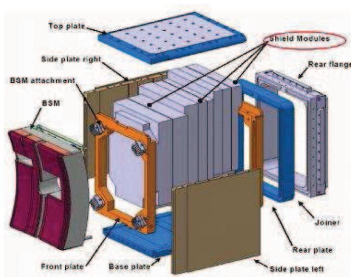
Figure 9.16. EPP details of ITER.
