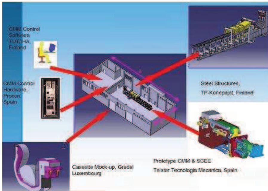
**Figure 9.3.** Layout and equipment of DTP-2 installation at Tampere,<sup>154</sup>. Dimensions (aprox.): a ≈ 50 m , b ≈ 20m.
