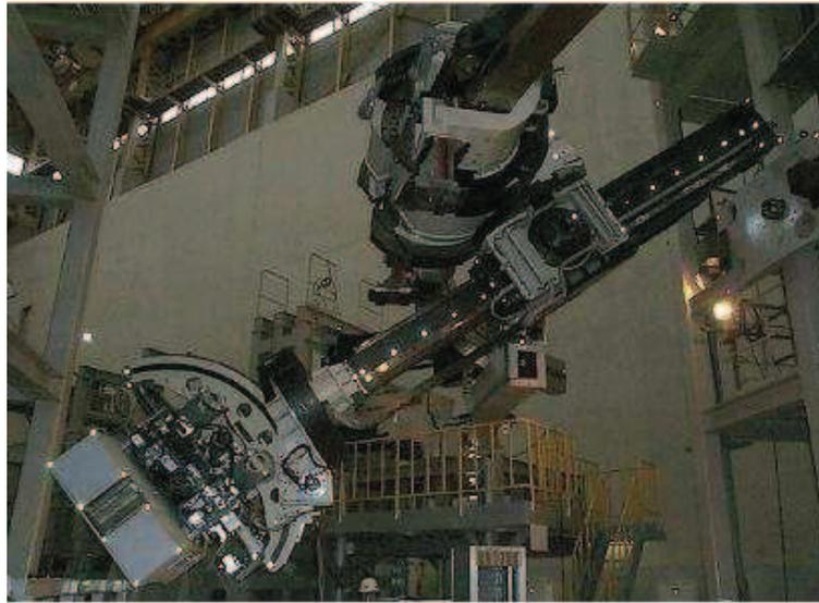
Figure 9.12. The vacuum vessel transporter.<sup>158</sup>
