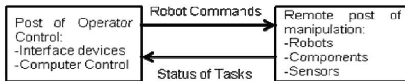
Figure 9.19. Scheme showing how a teleoperated system works.
