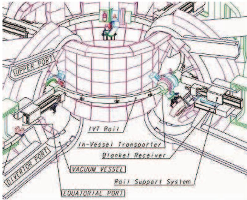
Figure 9.13. A schematic representation of the internal vacuum vessel in the interior of the ITER toroid.<sup>158</sup>
