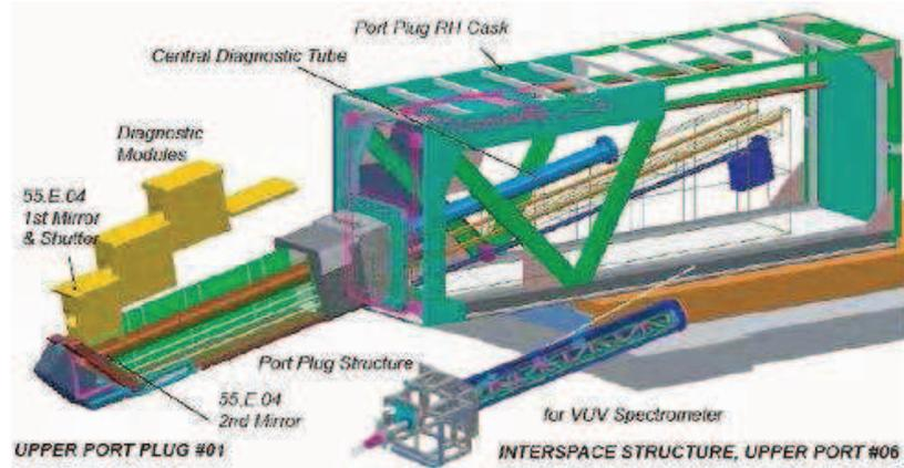
Figure 9.15. Details of an UPP of ITER.
