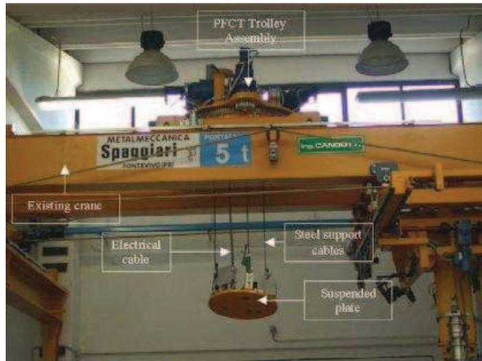
**Figure 9.7.** General view<sup>156</sup> of the Plasma Facing Components Transporter (PFCT). Assembly cart, cables, and suspended platform.
