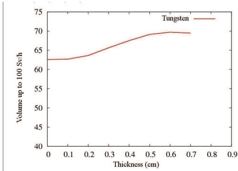
Figure II.6. Irradiated volume with dose rate between 100 and 500 Sv/h for a beam that sweeps the square area.
