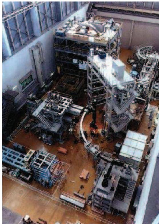
**Figure 9.11.** A general view of the Japanese IVT installation. The building is 30 m long and 10 m high. The semi-circle in the photograph is the 12 m diameter IVT rail <sup>158</sup>.
