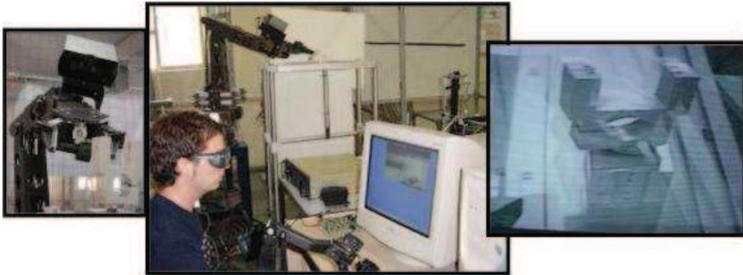
**Figure 9.21.** Stereoscopic Visualization System. Robot with binocular camera (left), operator with glasses for correct visualization of a stereoscopic image (centre), image of object as seen on the screen (right).
