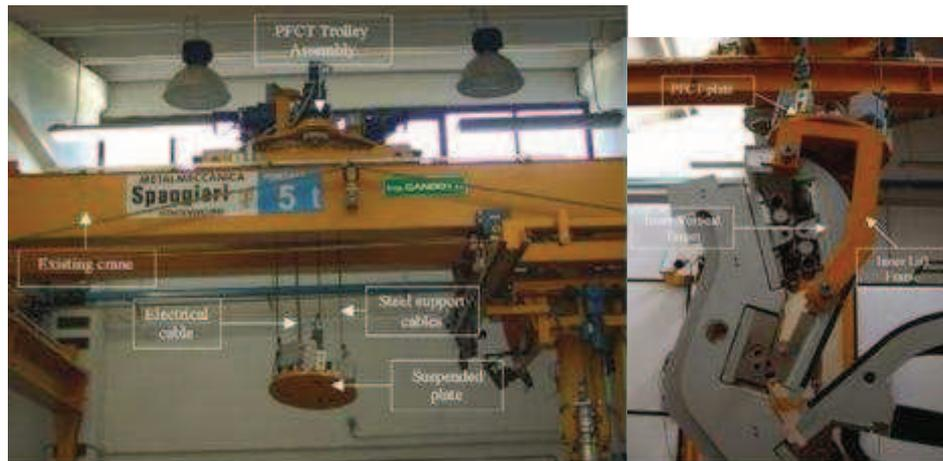
**Figure 9.25.** A general view of the component transporter from the first wall (PFCT). The principal elements of the PFCT are the trolley assembly, cables, and suspended disc (left). Part of the vertical corner of PFC (right).<sup>164</sup>.
