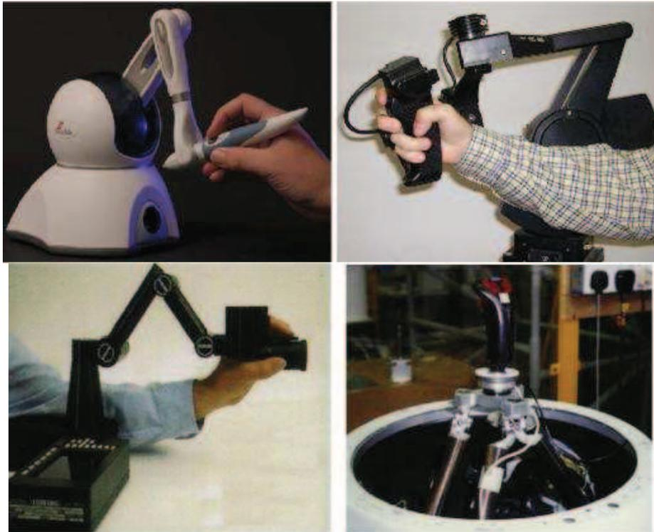
**Figure 9.20.** Different haptic devices used as masters for controlling remote robots Telemanipulation tasks.
