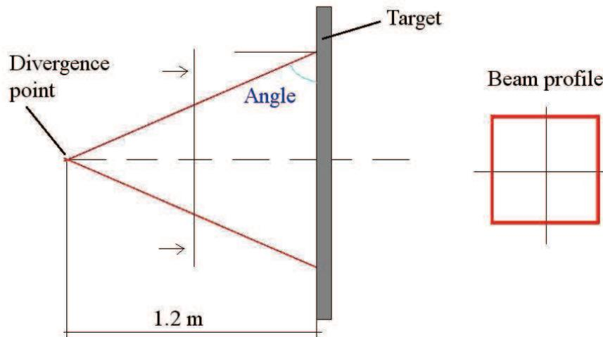
Figure II.2. Simulation model with the geometry introduced for the plate thickness calculation.
