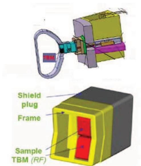
Figure 9.17. TBM structure for ITER.
