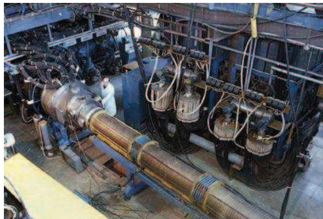
Figure 6.9. Photograph of the quasi-stationary plasma accelerator MK-200 (UG y CUSP), at the Troitsk Institute for Innovation & Fusion Research. Russia.
