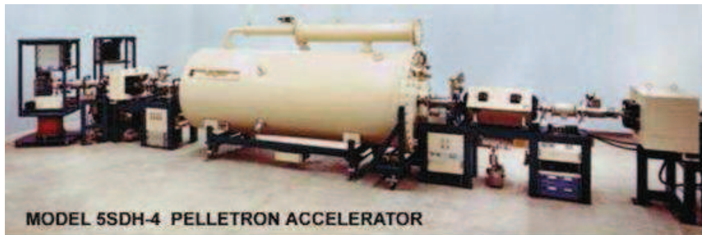
Figure 5.6. Tandem electrostatic accelerator 4 MV made by NEC.
